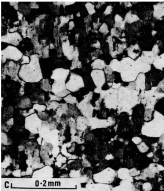
Fig. 2. Microstructures associated with the feldspars. (A) Recrystallized quartz enclosed by fine recrystallized albite. (B) Deformed muscovite (A) enclosing relic albites (B) and surrounded by fine recrystallized albite (C). (C) Deformed albite containing subgrains and recrystallized grains. (D) Deformed orthoclase, a zone of recrystallization occurs on the grain boundary adjacent to a biotite aggregate (B).
