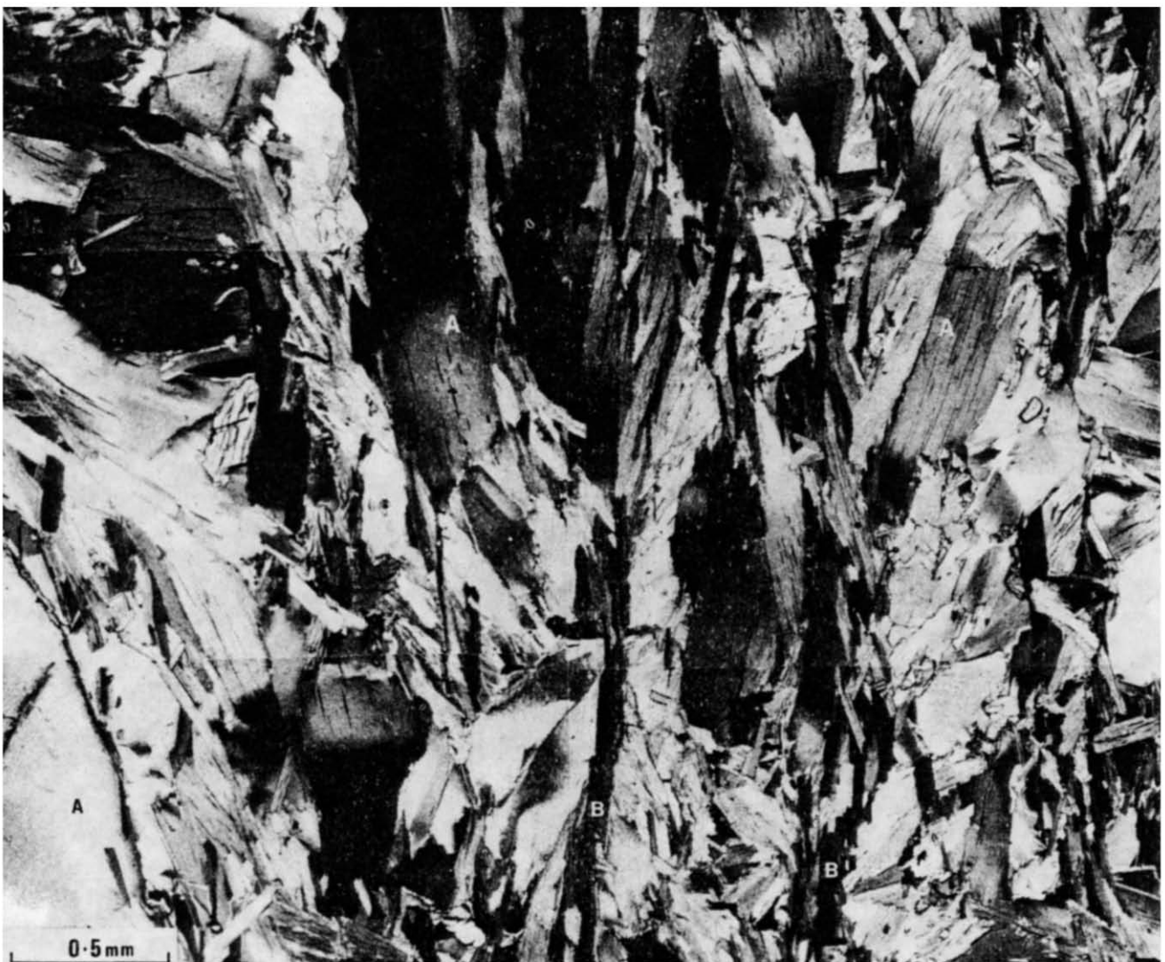
Fig. 4. Microstructural variation observed in a biotite aggregate intersected by a minor shear zone. Deformation is inhomogeneous and is controlled by the relative orientation of grains to one another and the concentration of other phases. A foliation is developed which is defined by an approximate parallelism of deformed pegmatitic biotites (A) and zones of metamorphic biotites (B).
